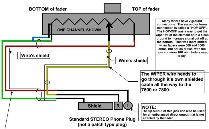
The TIP (Top of Fader) and the Ground should go through the same shielded wire and the shield should be grounded ONLY at the Plug
