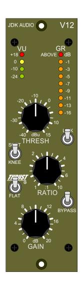
**NOTE:** Unlike the JDK R22 or other master/slave linked compressor pairs, where the master unit's control circuit becomes the master control for both units while the slave unit's controls are disabled, the V12 operates in a slightly different manner. Each V12 with the Link active will contribute their gain reduction
